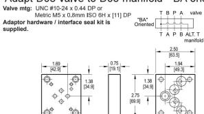
This adaptor permits the installation of a D03 valve on a D05 manifold. This adaptor, while low in cost, does not orient the A & B ports on the manifold to the respective valve solenoids.
